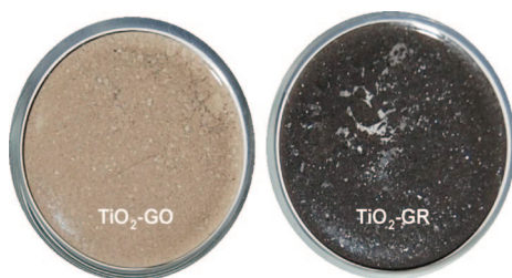
Figure 2. \text{TiO}_2 -graphene oxide ( \text{TiO}_2 -GO) and \text{TiO}_2 -reduced graphene ( \text{TiO}_2 -GR) powders obtained after solvent evaporation and drying the samples at room temperature.
